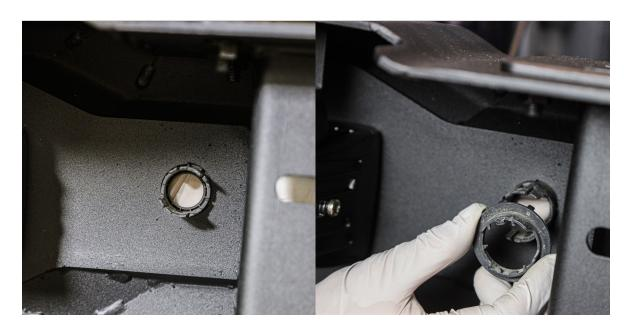
Follow the provided pictures to properly install the parking sensor housing. Ensure that the position and location of the sensors match those of your factory bumper, as mixing them up may result in error codes.
