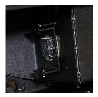
To secure them to the bumper, utilize **B07** bolts, **W11** washers, and **N09** nuts, employing a **10mm socket tool** and a **4mm hex tool**.
