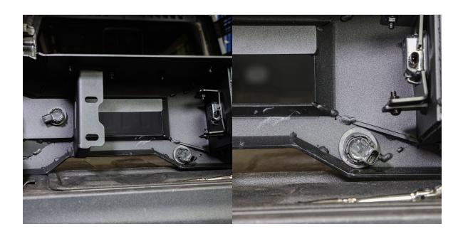
The bumper mounts to the frame using **B35** bolts, **W22** and **W23** washers, and **N15** nuts with a **16mm socket tool**.
