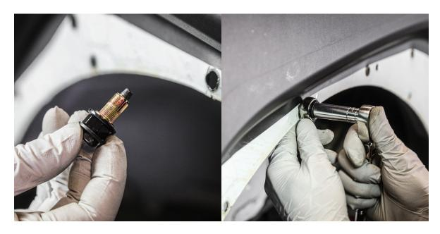
Drilling is necessary to fit the R01 rivet nuts into the holes.
