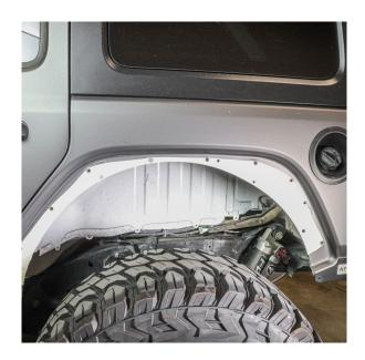
The mounting points require **B07** bolts and **W11** washers. Secure them using a **4mm hex tool**.
