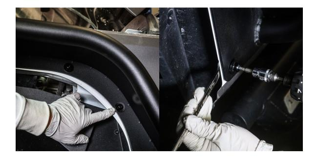
Secure them by fastening with a 5mm hex tool and a 10mm wrench. Make sure every mounting point is secured.
