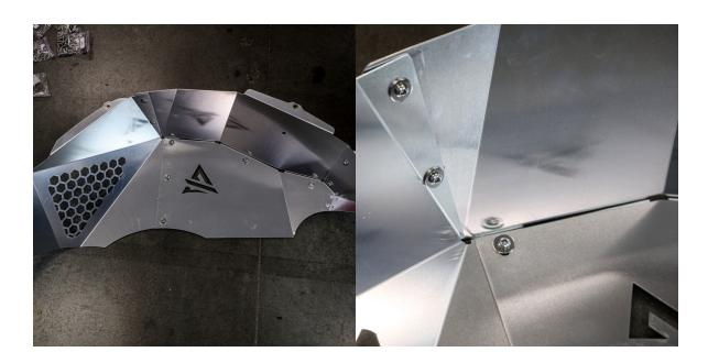
Preassemble the rear inner fender liner using **B60** bolts, **W08** and **W38** washers, and **N30** nuts. Leave the bolts finger tight, as they will be tightened in a later step.
