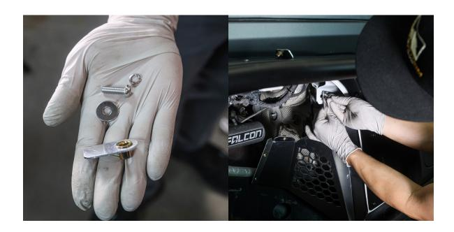
Secure the top mounting point using the threaded plate, **B61** bolts, **W38** washers, and **W08** washers. Use a **4mm hex tool** for this step. For the remaining mounting points, use **N30** nuts.
