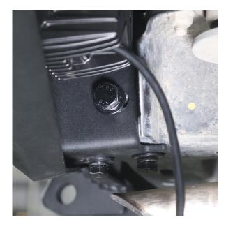
For the side mounting points, use **W35** and **W36** washers, and **B56** bolts with a **21mm** socket tool.
