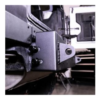
Once you are done hand-tightening the bolts on both sides of your rear bumper, it should mirror what is shown to the left.
