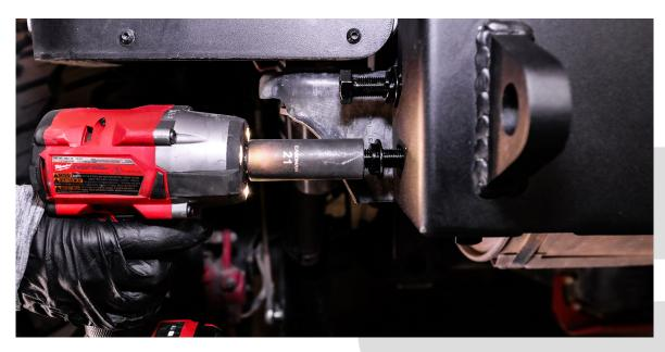
Once your **B37** bolts are tightened, continue with tightening the **B56** bolts on both sides of your rear bumper by using your **21mm Socket**.
