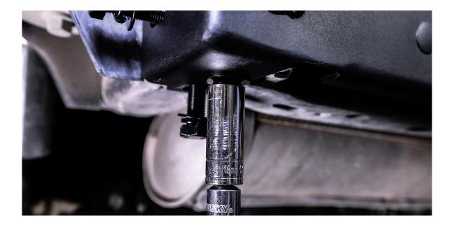
After all your bolts are hand-tightened. Proceed with tightening the **B37** bolts on both sides of the rear bumper with your **18mm Socket** to help your lift bumper into position. Please note: Use your **21mm Socket** for bottom **B56** bolt if needed.
