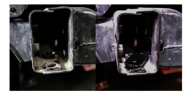
Please Note: Some model's of the Wrangler JL have a threaded insert located where your **threaded plate** should go. If so, do not panic, just flip your threaded plate over and only fasten the outermost nut as shown above.
