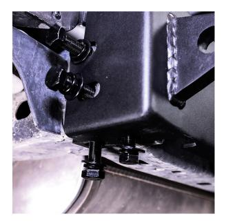
Please note: Some model's of the Wrangler JL have a threaded insert located where your **threaded plate** should go. If so you will need to proceed with using **B56** bolt, **W36** lock washer & **W35** washer in the same location where the threaded insert resides as shown on the right.
