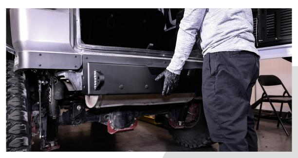
Once your **threaded plate(s)** are in position, proceed with inserting your rear bumper into place.
