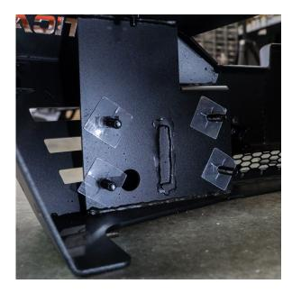
Insert **B34** bolts and **W21** plastic retainers onto the bumper as shown on the left.
