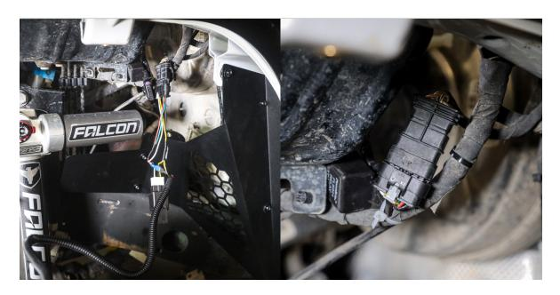
The front modular wing lights connect to your headlight harness. Install the Attica inline headlight harness adapter.
