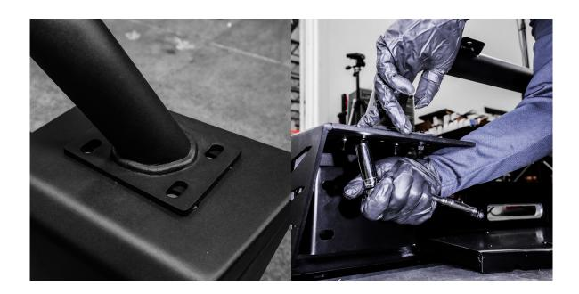
Align the mounting points of your bull bar with the top of your front bumper as shown above. It mounts to the front bumper using your **B19** bolts, **W19** washers and **N14** nuts with **5mm hex tool** & **13mm socket tool**.
