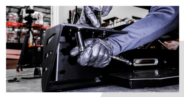
Next step is to slide your winch plate into the place behind the bumper.
