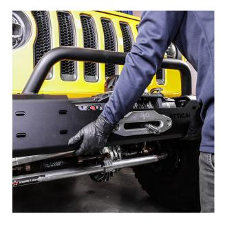
Once mounted, secure and fasten your D-Ring hooks on each side of the front bumper. Fasten with **B57** bolts, **W23** washers, **W22** lockwashers & **N15** nuts from behind the bumper with **16mm** socket tool & **16mm** wrench.
