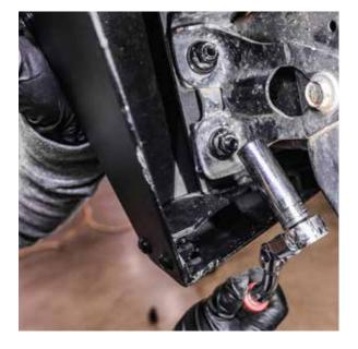
Secure by fastening your **W23** washers and **N17** nuts as shown on the left using your **16mm socket tool**.
