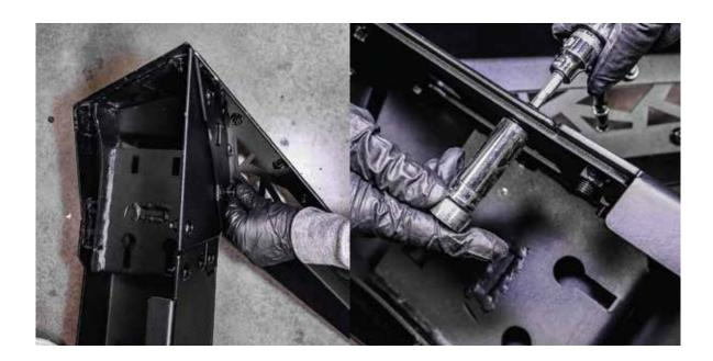
Align the mounting points of your bull bar with the top of your front bumper as shown above. After mounting to the front bumper using your **B15** bolts and securing by fastening your **N14** nuts on the underside using your **5mm hex tool** & **13mm socket tool**.
