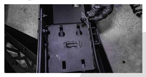
Once your bull bar is installed, flip your bumper so that the back is facing upwards, as shown above. Proceed by inserting your **square neck bolts** and **plastic retainers**.
