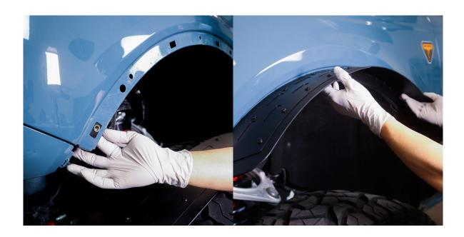
Align the squared mounting points of your vehicle's body with the **threaded plate**, as shown above. Then, mount the fender flare to the vehicle using the **threaded plate** along with **W09** and **W13** washers. Secure it in place by fastening the **B66** bolt using a **4mm hex socket tool**.
