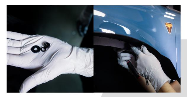
Attach the remaining mounting points using **W09** and **W13** washers, **N09** nuts, and **B66** bolts. Secure them in place by tightening with a **10mm wrench** and a **4mm hex socket tool**.
