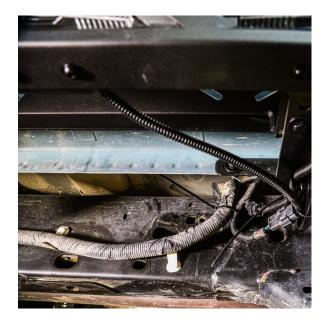
Secure the wiring harness using zipties.
