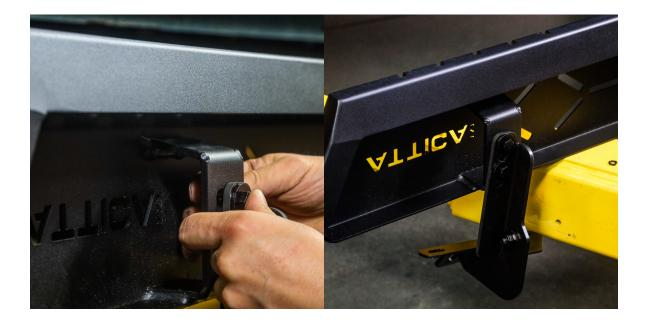
Attach the hardware support brackets to the side step using **B20** bolts, **W16** and **W19** washers, and **N22** nuts. Leave the hardware loose allowing movement in the bracket.
