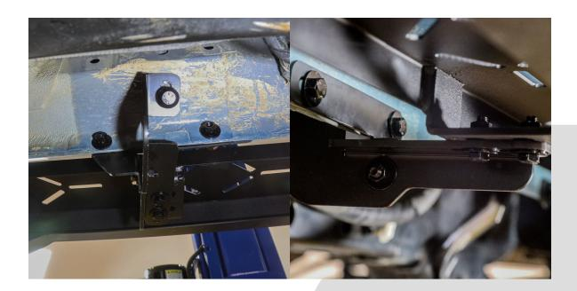
The side steps mount to your vehicle using **B32** bolts, **W22** and **W23** washers. For the smaller mounting points, use **B20** bolts, **W16** and **W19** washers, and **N22** nuts.
