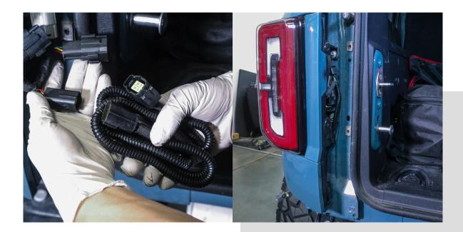
After completing the previous step, connect it to the other adapter(s). Once finished, feed the wire harness underneath so that it can be connected to the lights on the side step.
