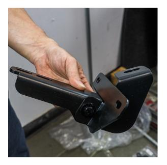
Start by installing the two hardware support brackets together using **B20** bolts, **W16** and **W19** washers, and **N22** nuts.
