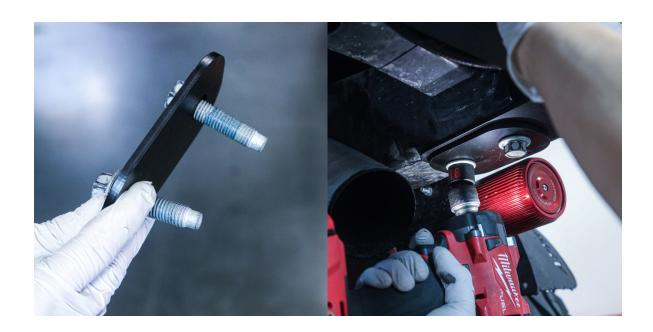
Use the factory bolts and Attica reinforcement plate, tighten four bottom bolts using an **18mm socket**.
