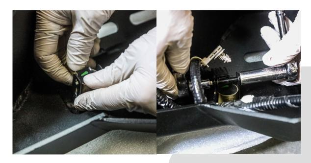
Attach the backup parking sensor to the rear bumper using a **B46** hex head bolt. Secure it in place with an **N09** nut and a **W25** washer, using a **4mm hex tool** and a **10mm socket**.
