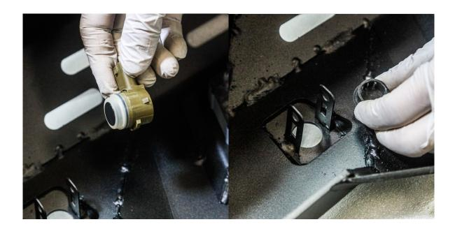
Remove your backup parking sensor from your factory rear bumper and locate the mounting point on the Attica Terra Series Rear Bumper.
