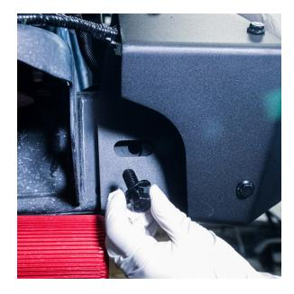
Use a **B37** bolt and a **W27** washer. Thread it into the nut on the L bracket using an **18mm socket**.
