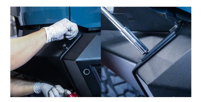
Attach the modular wing to the rear bumper using the **B22** bolts, and secure them by tightening a **13mm socket tool**.
