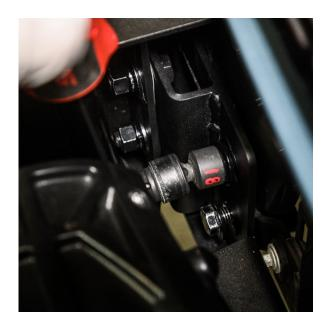
Once your bull bar is installed, mount your bumper using factory bumper bolts.
