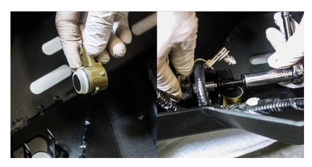
To install your parking sensors, use **N09** nuts and **B46** bolts securing them with a **4mm hex tool** and a **10mm socket**.
