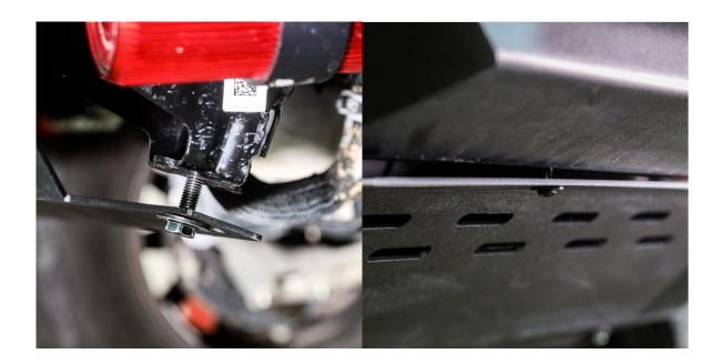
Installing each mounting point using W09 and W13 washers, and B07 bolts, secure them using a 4mm hex tool.
