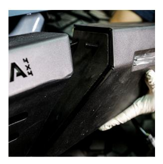
After reinstalling your headlights and grille, proceed to position the modular wing onto the bumper.
