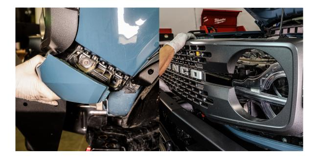
After removing the grille bolts, gently pull out a bit of the body panel to create enough space for removing the headlight bolts.
