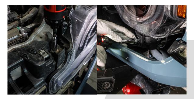
Locate and remove the three headlight bolts to take out your headlight.
