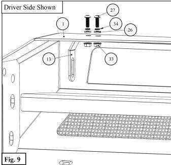
9. Loosely install the bumper assembly to the Mounting Brackets (5,6) using the supplied M12 Hardware. See **Figures 10 & 11.**
