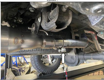
**STEP 8:**SLIDE A CLAMP ONTO THE LEFT TAILPIPE B AND INSTALL ONTO THE TAILPIPE A
