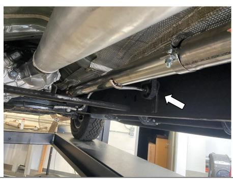
**STEP 2:** LOOSELY SECURE THE FRONT FLANGE PIPE TO THE OEM TAILPIPE.
