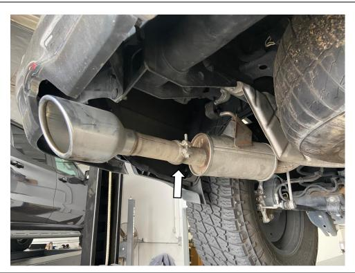
**STEP 2:** LOOSEN THE CLAMP FROM THE PASSENGER SIDE TAILPIPE AND REMOVE FROM VEHICLE.
