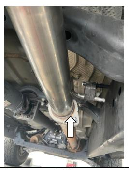
STEP 2: SLIP A CLAMP ON THE FLANGE PIPE AND THEN INSTALL THE MUFFLER. SUPPORT THE MUFFLER WITH A STAND. SNUG CLAMP BUT LEAVE LOOSE FOR ADJUSTMENTS LATER. POSITION MUFFLER WITH LOGO FACE DOWN.
