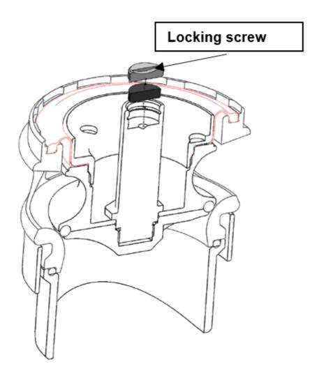
Inspect for Damage before inserting piston assembly into Raceport Body. Ensure Diaphragm bead is seated correctly in the groove on the body.
