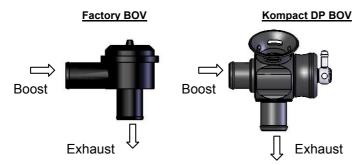
**NOTE:** Be sure to mount the Kompact Dual Port in the orientation shown above compared to the standard BOV.
