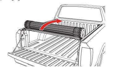
Fold the front panel back and insert the two mounting bolts (K) into the slotted bracket. Do this for both sides. The bolts will align with the slotted bracket of the cover rail. Fold the panel back down.
