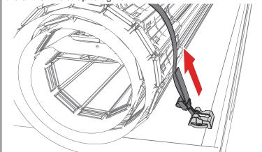
**CLOSING COVER:** Roll the cover (E) toward the tailgate and rotate the tail rail downwards towards the rotating locking
