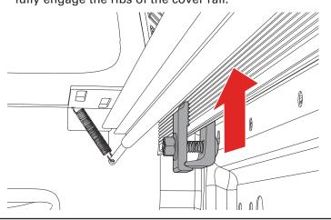
Mount the strap clamp assembly (F) as far forward as possible. Hand tighten to 10 ft/lbs of torque with a 9/16" wrench or socket. Apply downward pressure to the cover rail when tightening the clamps to ensure that the rail sits flush and the seals are set.
