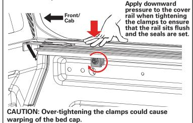
**NOTE**: When installing each clamp (G), make sure that the clamps are inserted as far up onto the rail as possible and that the clamp teeth fit squarely and fully engage the ribs of the cover rail.
