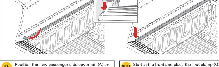
Position the new passenger side cover rail (A) on the truck rail with the slotted bracket pushed all the way toward the front/cab and the bulkhead.
