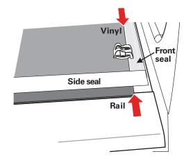
Verify that a gap of approximately 1/8" (3.2mm) remains on both sides of the cover (E) between the edge of the cover rail and the rolling cover. This spacing is necessary to ensure that the locking rail secures to cover. Align the cover side to side at the front and/or the back if the side gaps are not even. Firmly hand tighten the knobs (H) after the cover has been aligned.
