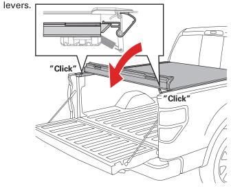
**OPENING COVER:** Pull down on the latch release cable located on either side of the cover (E) and rotate the tail rail forward and into a rolling motion. When driving with the cover open, the cover must be rolled toward the cab and secured with **BOTH** strap clamps.
