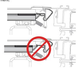
When the rolled cover (E) is properly aligned, roll it open, ensuring not to misalign while opening. Tighten the knobs (I) on both sides to secure the cover. **DO NOT overtighten**. Hand tighten only. Recheck that the cover operates correctly. Close the cover and check that the locking levers are engaged and prevent the hard rolled cover from being lifted on both sides.
