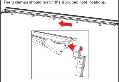
Mount the passenger side rail (A) into the holes in the truck bed. Reuse the screws from step 6, using a drill/socket wrench. Before tightening, make the necessary adjustments for the rail so that it has proper clearance to both the front cargo rail and the tailgate. Make sure the passenger side rail is pushed tight up against the front cargo rail.
