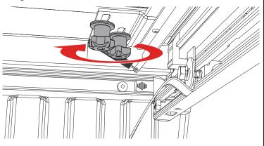
When the cover (E) is in the open position, the other end of the strap clamp assembly (N) inserts into the cover clasp and turns to lock. Pull up on the strap end to tighten. Always hook the straps on BOTH sides.
