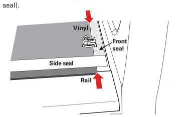
Verify that a gap of approximately 1/8" (3.2mm) remains on both sides of the rolled cover (E) between the edge of the cover rail and the rolling cover. This spacing is necessary to ensure that the locking rail secures to cover. Align the cover side to side at the front and/or the back if the side gaps are not even. Firmly hand tighten the knobs (I) after the cover has been aligned.
