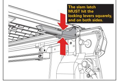
Check to see that the latches on both sides at the tailgate fully engage the cover rails (A & B). Loosening the lock knobs (I) and making the side to side adjustment as in step 18 could help with the latch striker engagement.
