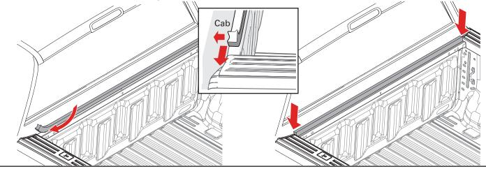
Align the S clamps (G) with the passenger side rail slot and insert into the new passenger side cover rail (A).
