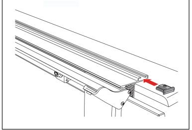
**ROLLED UP POSITION:** To drive with the cover (E) in the open position, use the strap clamps. Roll the cover forward, twist and insert the clips into the cover clasps. Ensure that BOTH strap clamps are fully inserted into the clasps. Pull on the end of the strap to tighten.
