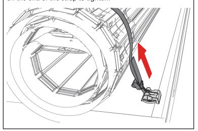
**CLOSING COVER:** Roll the cover (E) toward the tailgate and rotate the tail rail downwards towards the rotating locking levers.
