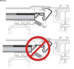
When the rolled cover (E) is properly aligned, roll it open, ensuring not to misalign while opening. Tighten the knobs (I) on both sides to secure the cover. **DO NOT overtighten**. Hand tighten only. Recheck that the cover operates correctly. Close the cover and check that the locking levers are engaged and prevent the hard rolled cover from being lifted on both sides.
