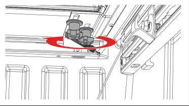
When the cover (E) is in the open position, the other end of the strap clamp assembly (N) inserts into the cover clasp and turns to lock. Pull up on the strap end to tighten. Always hook the straps on BOTH sides.
