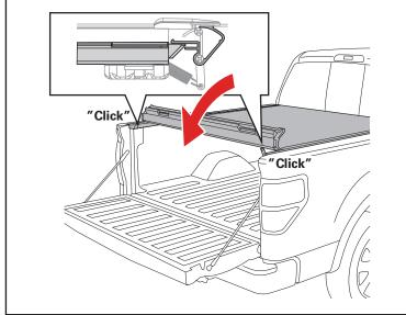
**OPENING COVER:** Pull down on the latch release cable located on either side of the cover (E) and rotate the tail rail forward and into a rolling motion. When driving with the cover open, the cover must be rolled toward the cab and secured with **BOTH** strap clamps.
