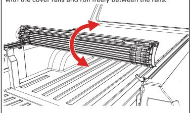
Align the front vinyl edge of the rolled cover (E) with the front edge of the side rails (not the rubber
