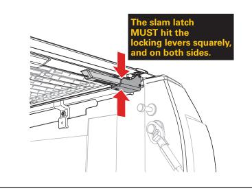
Check to see that the latches on both sides at the tailgate fully engage the cover rails (A & B). Loosening the lock knobs (I) and making the side to side adjustment as in step 18 could help with the latch striker engagement.
