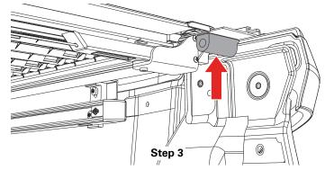
With both rails (A & B) clamped in place, rest the rolled cover (F) onto the rails at the tailgate, roll the cover toward the cab, and remove and discard all packaging materials.
