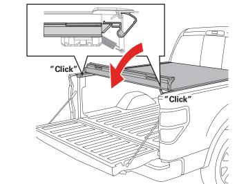
**OPENING COVER:** Pull down on the latch release cable located on either side of the cover (F) and rotate the tail rail forward and into a rolling motion. When driving with the cover open, the cover must be rolled toward the cab and secured with **BOTH** strap clamps.
