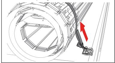
**CLOSING COVER:** Roll the cover (F) toward the tailgate and rotate the tail rail downwards towards the rotating locking levers.
