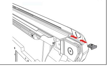
**ROLLED UP POSITION:** To drive with the cover (F) in the open position, use the strap clamps. Roll the cover forward, twist and insert the clips into the cover clasps. Ensure that BOTH strap clamps are fully inserted into the clasps. Pull on the end of the strap to tighten.
