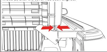
When correctly installed, the vinyl edges of the rolled cover (F) will align squarely with the side rails in all four corners. The latch assembly will align with the side rail locking levers at the tailgate on both sides.
