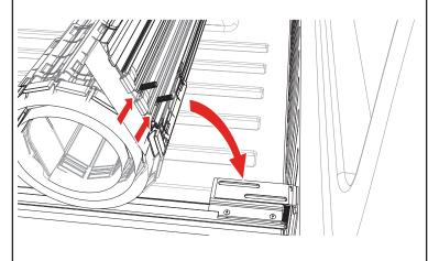
Install the mounting hardware from step 2 loosely underneath the slotted bracket on the passenger rail. Start with the rubber washer (L), then the large flat washer (K), then hand tighten the knobs (J). Repeat on the driver's side. Leave the knobs loose for now.
