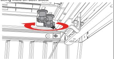
With the cover in the open position, the other end of the strap clamp assembly (G) inserts into the cover clasp and turns to lock. Pull up on the strap end to tighten.
