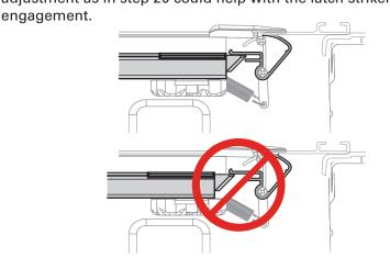
When the rolled cover (F) is properly aligned, roll it open, ensuring not to misalign while opening. Tighten the knobs (J) on both sides to secure the cover. **DO NOT overtighten**. Hand tighten only. Recheck that the cover operates correctly. Close the cover and check that the locking levers are engaged and prevent the hard rolled cover from being lifted on both sides.
