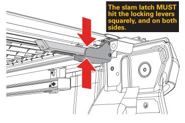
Check to see that the latches on both sides at the tailgate fully engage the cover rails (A & B).
