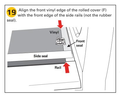
Verify that a gap of approximately 1/8" (3.2mm) remains on both sides of the rolled cover (F) between the edge of the cover rail and the rolling cover. This spacing is necessary to ensure that the locking rail secures to cover. Align the cover side to side at the front and/or the back if the side gaps are not even. Firmly hand tighten the lock knobs (J) after the cover has been aligned.
