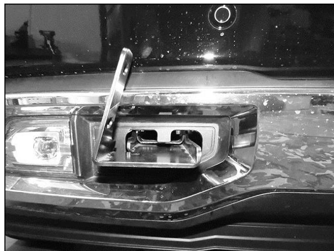
(Fig 11) Passenger/right side Bracket installed
