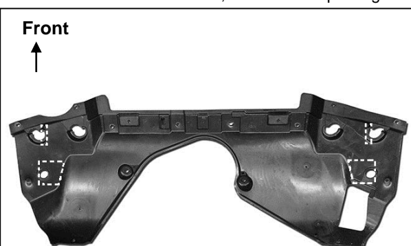
(Fig 11) Hold splash guard up to bottom of Brackets to determine areas to cut from cover. (Bottom of splash guard pictured)
