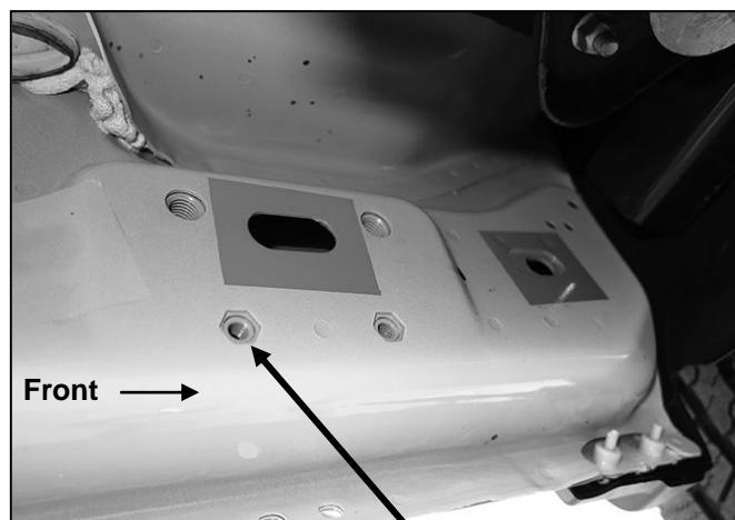
(Fig 9) Driver side front mid 2015-on, an example of models with factory installed threaded inserts
