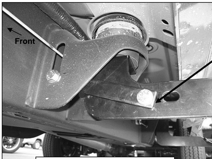
(Fig 6) 1500 Model Center Support Bracket Installation Pictured
