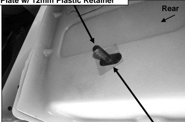
(Fig 12) Try to keep the Bolt Plate in the center of the slot when installing the rear Bracket only
