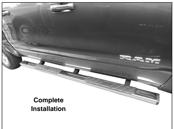
(Fig 7) Passenger/right Sidebar attached to Mounting Brackets at the center and rear locations
