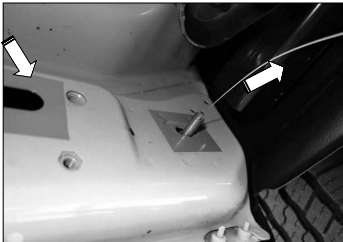
(Fig 3) With the 10mm Bolt Plate attached, slowly pull the Fish Wire back through the forward hole in the body panel. Once completely exposed as pictured, firmly hold the Bolt Plate in place, remove the Fish Wire and thread (1) 10mm Plastic Retainer onto the Bolt Plate to hold it in place (see Fig. 5),
