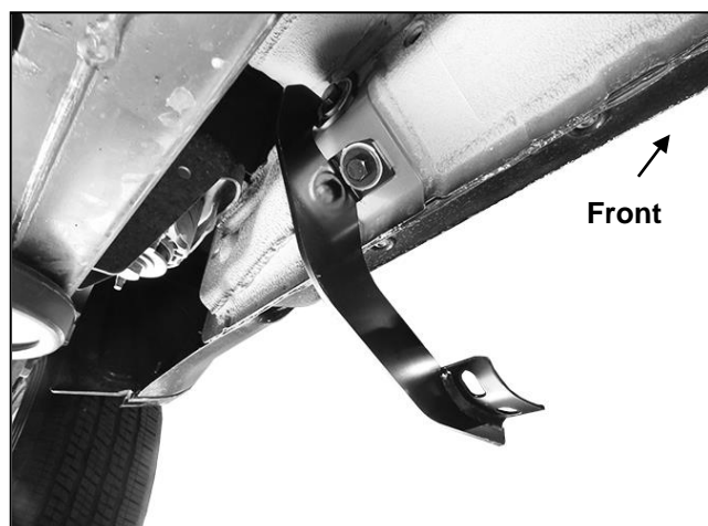
(Fig 7) Driver/Left Rear Mounting Bracket installed
