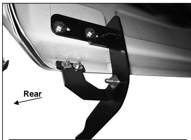
(Fig 16) Driver/Left rear Brackets installed
