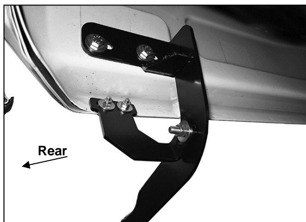
(Fig 14) Driver/Left rear Brackets installed
