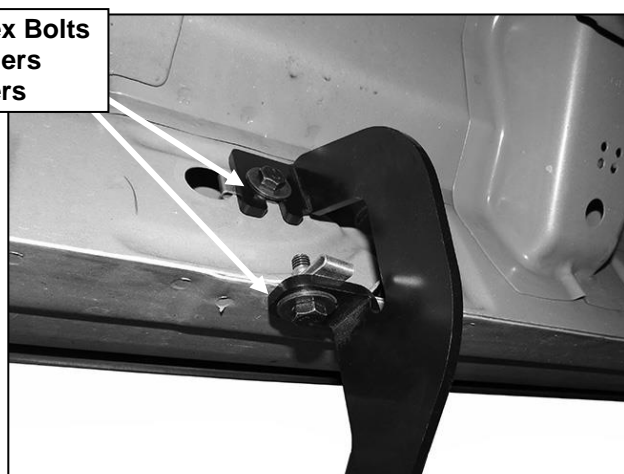
(Fig 7) Example of Bracket bolted to 8mm Clip Nuts on mounting tab and inner body panel
