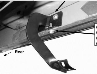
(Fig 3) Driver side-rear Mounting Bracket location
