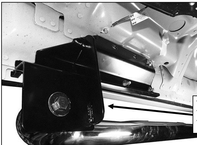
(Fig 5) Passenger side front Bracket installation
