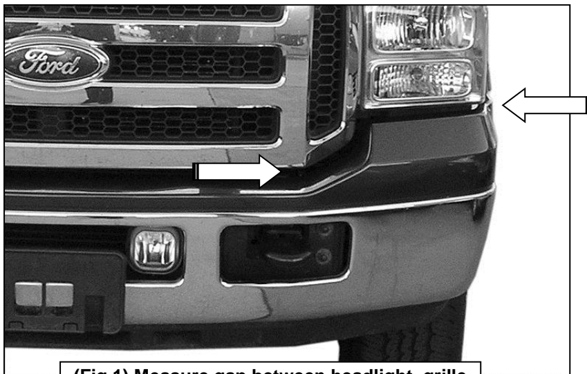
(Fig 1) Measure gap between headlight, grille and bumper before loosening bumper bolts
