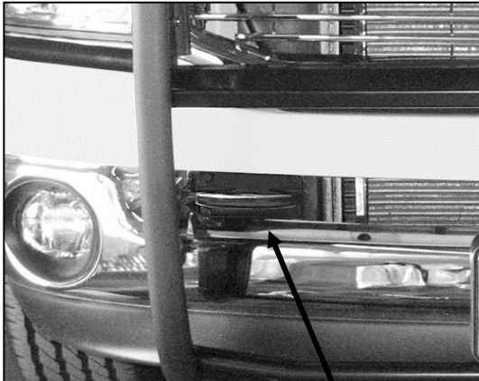
(Fig 8) Grille Guard mounted with factory tow hook. Use the supplied longer: 10mm x 45mm Hex Bolts 10mm Flat Washers 10mm Nylon Lock Nuts for tow hook installation
