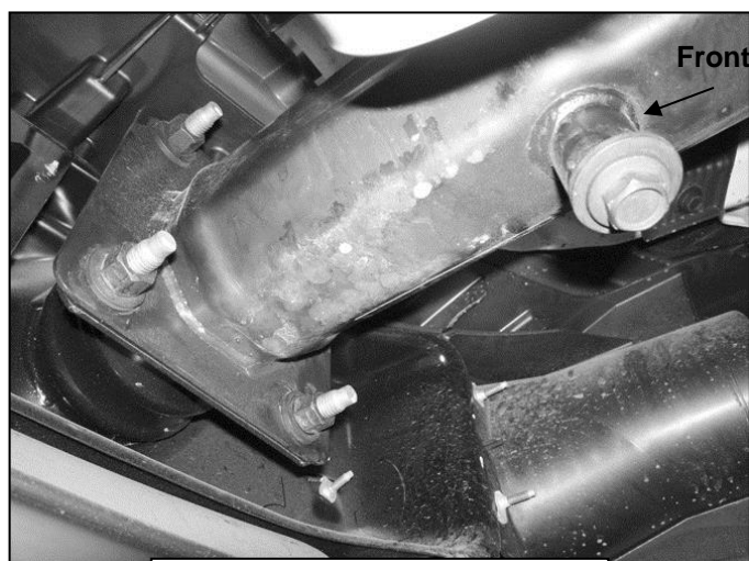
(Fig 1) Passenger side bumper bracket pictured from below. Remove (2) bottom flange nuts
