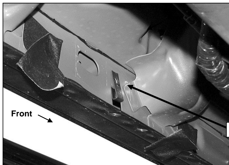
(Fig 4) Driver side-center Mounting Bracket location
