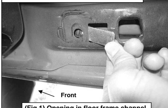
(Fig 1) Opening in floor frame channel (passenger side-front pictured)
