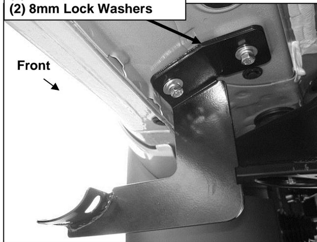
(Fig 2) Driver side front mounting location pictured
