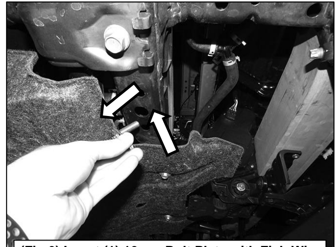
(Fig 6) Insert (1) 10mm Bolt Plate with Fish Wire into the large hole on the crossmember and out the smaller hole towards the side of the vehicle
