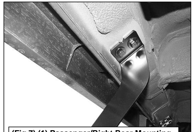
(Fig 7) (1) Passenger/Right Rear Mounting Bracket attached to the 2nd location
