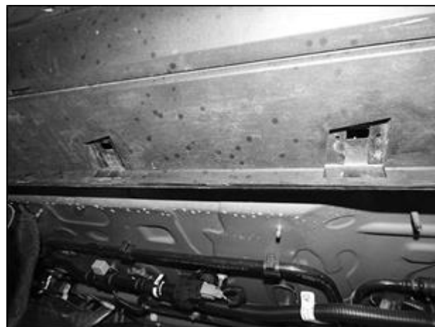
(Fig 13) Insert (2) 10mm Spiral Bolts into the outer center location
