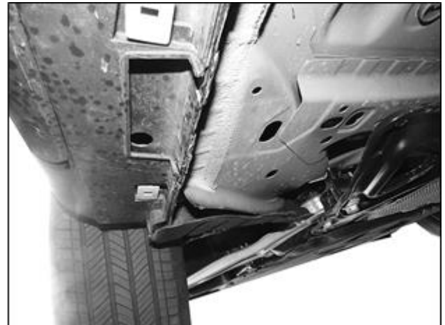
(Fig 4) Locate the Driver/Left front mounting location
