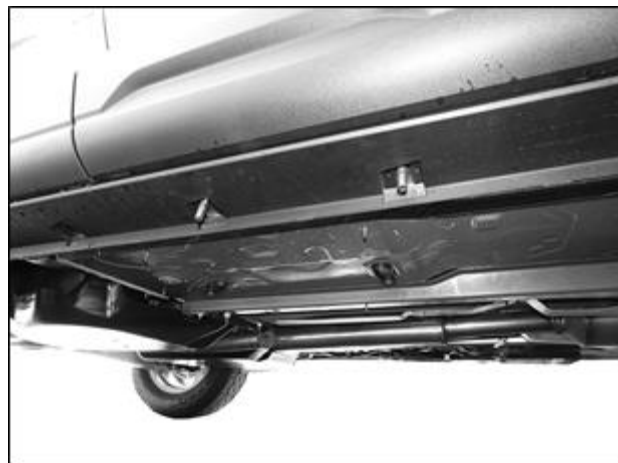
(Fig 14) (2) 10mm Spiral Bolts inserted into the outer center location
