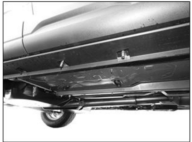
(Fig 11) (2) 10mm Spiral Bolts inserted into the outer center location
