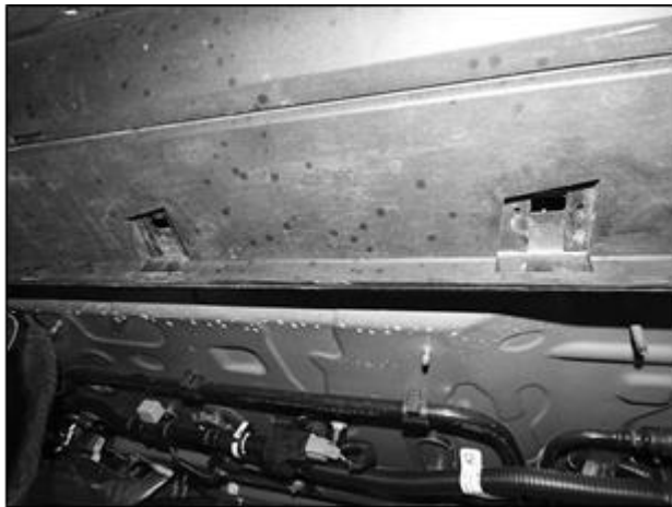
(Fig 10) Insert (2) 10mm Spiral Bolts into the outer center location
