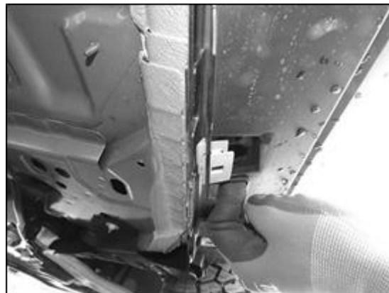
(Fig 2) Gently pull the trim slightly to loosen the clips (Passenger side shown)
