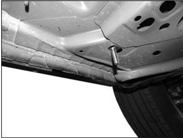
(Fig 6) Insert (1) 10mm Short Bolt Plate into the floor panel
