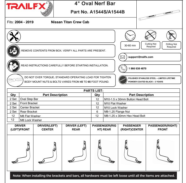
**1.** Remove all contents from the package and check stainless steel tubes for any damage. Also, verify that all components and hardware listed above are included before you begin installation.
